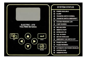
**Description**—Firetrol\* FTA1800 Autotransformer Starting Fire Pump Controllers use an autotransformer to supply reduced voltage when starting the motor. The controller is of the closed circuit type where the motor circuit remains closed during the transition from start to run resulting in minimum line disturbance.
